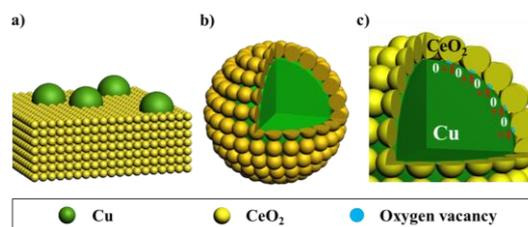
**Scheme 1.** Schematic illustration of a) Cu/CeO<sub>2</sub>-IM prepared by conventional impregnation method, b) Cu@CeO<sub>2</sub> fabricated by the facile sol-gel method, c) Cu<sup>0</sup> and Cu<sup>+</sup> distribution of the reduced Cu@CeO<sub>2</sub> catalyst.
