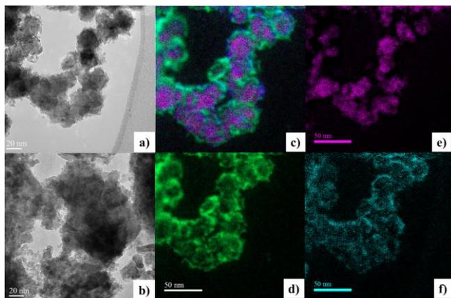
**Figure 1.** TEM images of the reduced a) 30Cu@CeO<sub>2</sub> and b) 30Cu/CeO<sub>2</sub>-IM; the corresponding EELS spectrum imaging of the reduced 30Cu@CeO<sub>2</sub>: c) the composite image, d) the Ce-M edge map, e) the Cu-L edge map and f) the O-K edge map.
