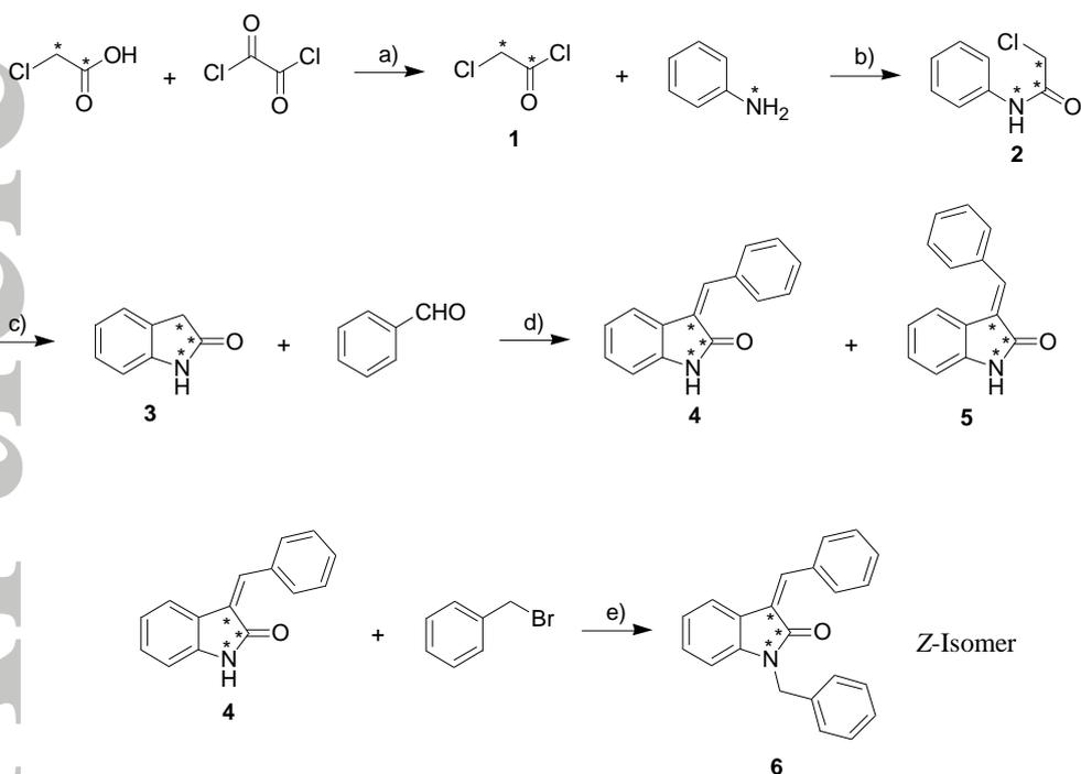
**SCHEME 1** Synthesis of [ $^{13}\text{C}_2$ ,  $^{15}\text{N}$ ]-1,3-2*H*-1-benzyl-(*Z*)-3-(benzylidene)indolin-2-one
