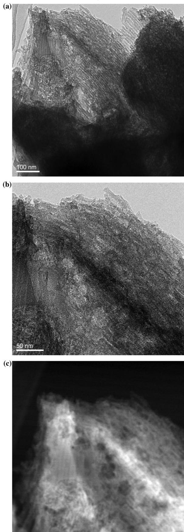
**FIGURE 2** a-b) TEM images and c) HAADF image of Cu NPs-MCN nanocomposite
