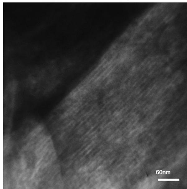
**FIGURE 6** TEM image of cu NPs-MCN reused after eight cycles in multicomponent 1,3-dipolar cycloaddition between of benzyl bromide, phenylacetylene and sodium azide
