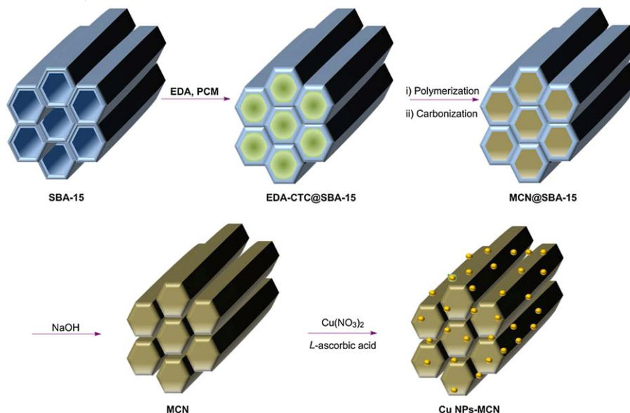
**SCHEME 1** Schematic illustration of Cu NPs-MCN nanocomposite preparation
