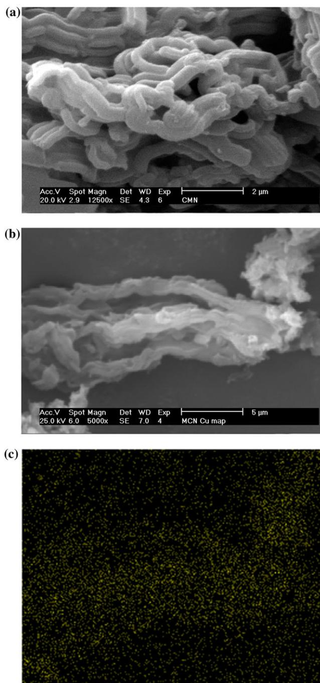
**FIGURE 1** SEM images of a) MCN and b) Cu NPs-MCN nanocomposite; c) corresponding quantitative EDS element mapping of Cu
