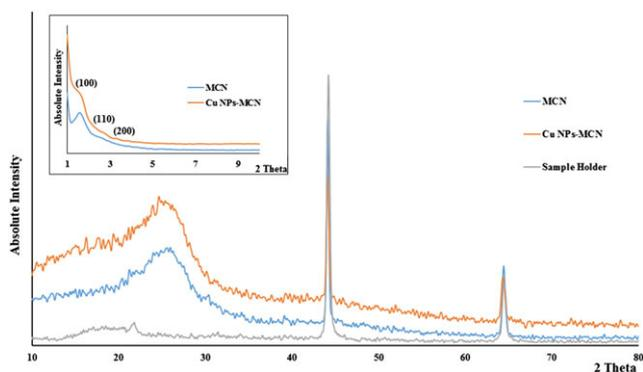
**FIGURE 4** The high angle XRD patterns of MCN and cu NPs-MCN (inset: Low angle)
