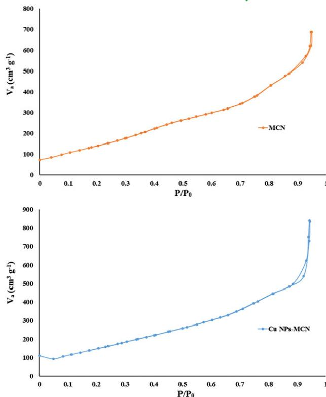
**FIGURE 5** Nitrogen adsorption/desorption isotherms of MCN and cu NPs-MCN
