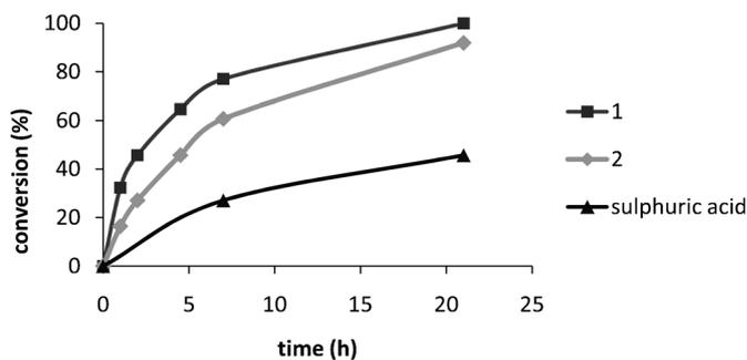
**Figure 2.** Sunflower seed oil transesterification with 1 wt% sulphuric acid and the same molar amounts of Twitchell reagents **1** and **2**. The molar ratio methanol to triglyceride was kept at 6/1 and the temperature at 60 °C.
