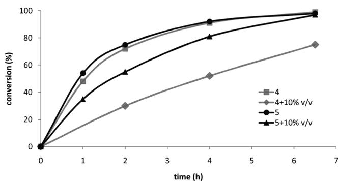
**Figure 8.** Sunflower seed oil transesterification with catalysts **4** and **5**, in the presence of methanol containing 0, 10% (v/v) of water. The molar ratio methanol to triglyceride was kept at 6/1 and the temperature at 60 °C.
