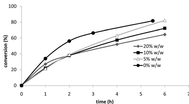
**Figure 7.** Sunflower seed oil transesterification with catalyst **4**, in the presence of oil containing 5, 10, 20% (w/w) of stearic acid. The molar ratio methanol to triglyceride was kept at 6/1 and the temperature at 60 °C (FAME integral was used to measure the conversion).
