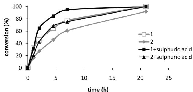
**Figure 3.** Sunflower seed oil transesterification with Twitchell reagents **1** and **2**, in the presence and absence of 1 wt% sulphuric acid. The molar ratio methanol to triglyceride was kept at 6/1 and the temperature at 60 °C.
