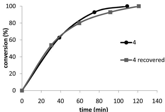
**Figure 12.** Sunflower seed oil transesterification catalysed by 18.5 wt% of compound **4** and catalyst **4** recovered. The molar ratio methanol to triglyceride was kept at 6/1 and the temperature at 80°C.
