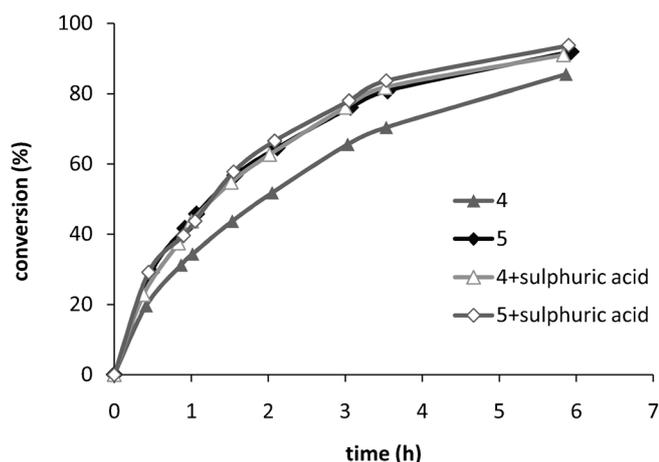
**Figure 6.** Sunflower seed oil transesterification with catalysts **4** and **5**, in the presence and absence of 1 wt% sulphuric acid. The molar ratio methanol to triglyceride was kept at 6/1 and the temperature at 60 °C.
