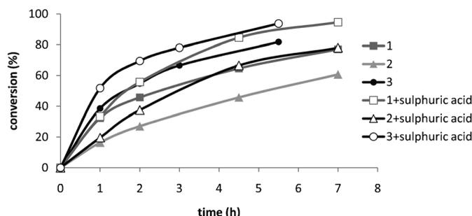
Figure 5. Sunflower seed oil transesterification with Twitchell reagents **1** and **2** and catalyst **3**, in the presence and absence of 1 wt% sulphuric acid. The molar ratio methanol to triglyceride was kept at 6/1 and the temperature at 60 °C.
