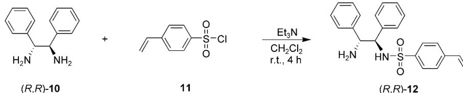
**Scheme 1.** Synthesis of chiral 1,2-diamine monosulfonamide monomer (*R,R*)-**12**.
