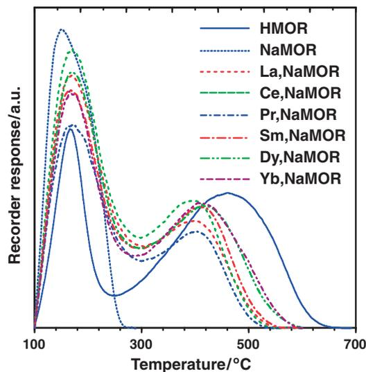
Figure 3.  $\text{NH}_3$ -TPD profiles of  $\text{Ln,NaMORs}$ .
