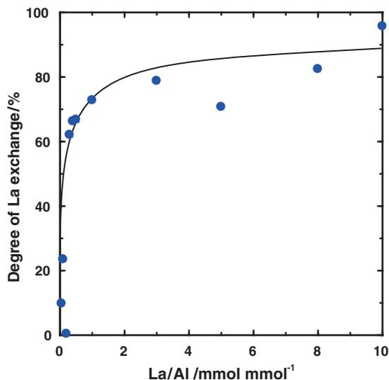
**Figure 1.** Effects of cation exchange on the lanthanum amounts against Al content of La,NaMOR.
