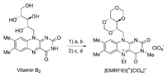
**Scheme 1.** Synthesis of [DMRFIEt]<sup>+</sup>[ClO<sub>4</sub>]<sup>-</sup>: a) HCHO, HCl, 60 °C, 3 days; b) CH<sub>3</sub>I, K<sub>2</sub>CO<sub>3</sub>, DMF, RT, overnight; c) CH<sub>3</sub>CHO, NaBH<sub>3</sub>CN, Na<sub>2</sub>S<sub>2</sub>O<sub>4</sub>, DMF, 60 °C, 2 h; d) NaNO<sub>2</sub>, HClO<sub>4</sub>, NaClO<sub>4</sub>, 0 °C.
