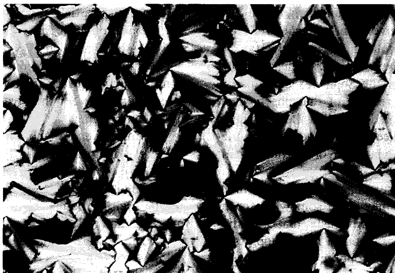
Fig. 1. The texture of the smectic A phase of octyl 1-thio- \beta -D-galactopyranoside at 137 °C upon cooling from the isotropic melt.
