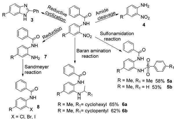
the differently protected *o*-phenylenediamine. *o*-Nitroanilides are known to be potential precursors for reductive cyclization to obtain 2-substituted benzimidazoles. 2-Amino-anilides can also be accessed from the reduction of the nitro compounds and later easily decorated with halogens by the Sandmeyer reaction.
