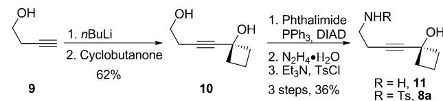
Scheme 2. Synthesis of model substrate **8a**.
