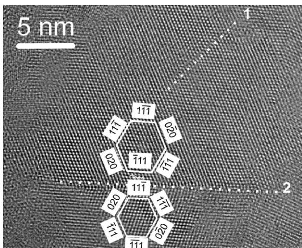
**Figure 2** Cross sectional HRTEM image along the [110] zone axis of the structure. Line 1 shows a stacking fault. Two Si-nc crystallites form a twin boundary located along line 2.
