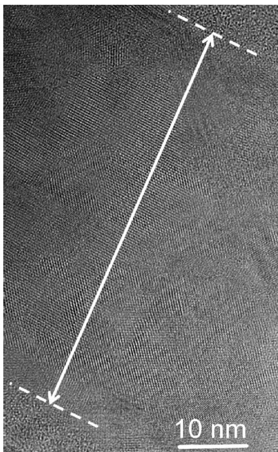
**Figure 1** Cross-sectional HRTEM image from crystallized Si film. Location and direction of the film is indicated with double-sided arrow and with dotted lines.
