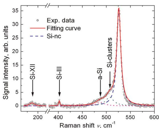
**Figure 3** (online colour at: www.pss-a.com) Raman spectrum detected from the crystallized Si film. The experimental data points were fitted with peaks related to Si-nc, Si-clusters (Si-nc precursors with dimensions <math><1\text{ nm}</math>), a-Si and high pressure Si phases, i.e. Si-XII and Si-III.
