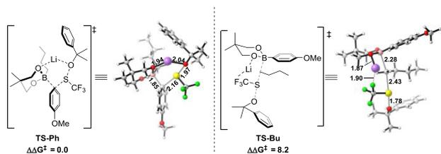
**Figure 5.** Computed transition state structures for aryl and alkyl trifluoromethylthiolation and their relative free energies in kcal/mol using the (SMD)-B3LYP-D3(BJ)/6-311+G(2d,p)/(SMD)-M06-2X/6-31G(d,p) method.
