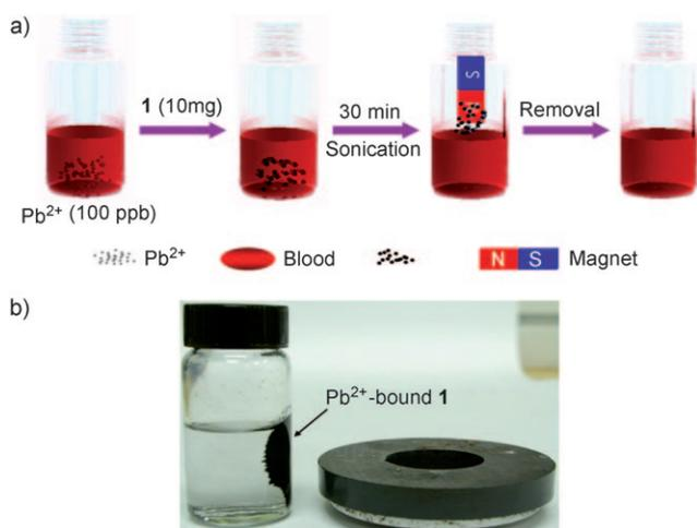
**Figure 5.** a) Illustration of the removal of Pb<sup>2+</sup> from human blood. b) Photograph of a magnet attracting Pb<sup>2+</sup>-bound **1** in water.
