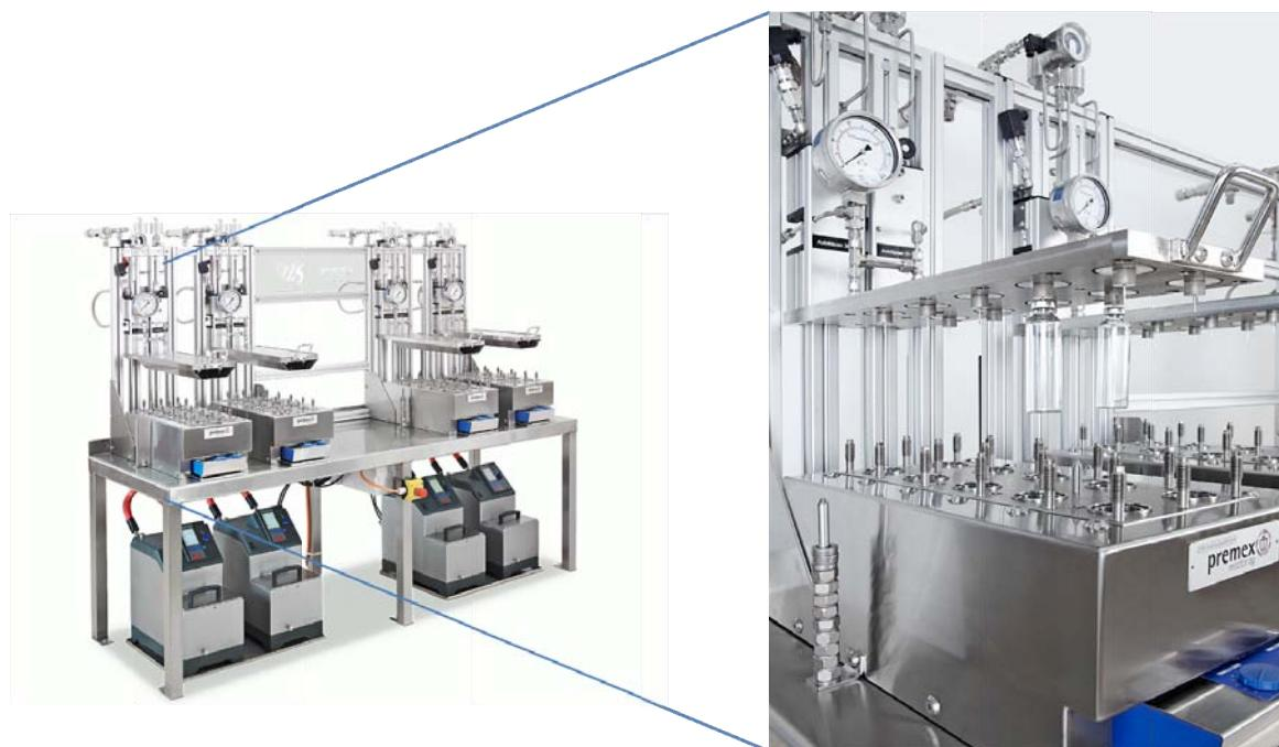
**Fig. (1).** Reactor set-up used for the high throughput experiments. Courtesy of ILS.
