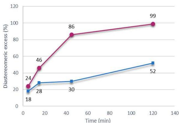
**Figure 1.** Evolution of the d.e. over time for 1 equivalent (blue curve) or 2 equivalents (pink curve) of P<sub>4</sub>t-Bu (<sup>19</sup>F NMR study)
