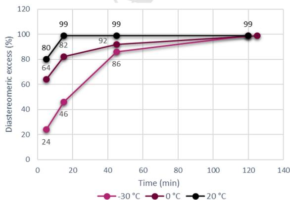
**Figure 2.** Evolution of the diastereomeric excess over time at different temperatures for 2 equivalents of P<sub>4</sub>t-Bu (<sup>19</sup>F NMR study)
