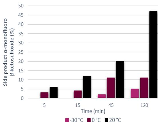
**Figure 3.** Evolution of the percentage of side products **22a** formed over time at different temperatures for 2 equivalents of P<sub>4</sub>t-Bu (<sup>19</sup>F NMR study)
