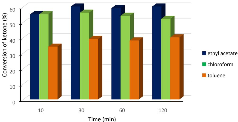
**Figure 1.** The influence of the solvent type on the conversion of ketone in chemo-enzymatic Baeyer-Villiger oxidation carried out in the flow reactor. All experiments were performed in triplicate and the results for each of the three measurements differed by less than 1%.
