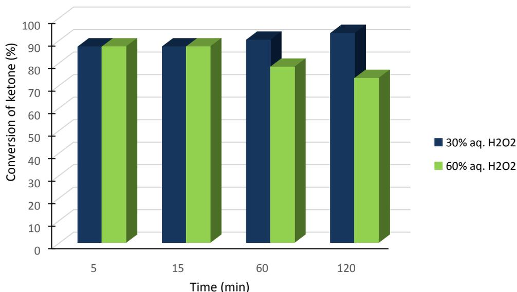
**Figure 3.** The influence of the H<sub>2</sub>O<sub>2</sub> concentration on the conversion of ketone in chemo-enzymatic Baeyer-Villiger oxidation carried out in the flow reactor. all experiments were performed in triplicate and the results for each of the three measurements differed by less than 1 %.
