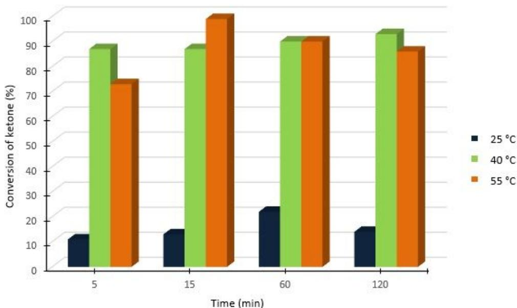
**Figure 2.** The influence of the temperature on the conversion of ketone in chemo-enzymatic Baeyer-Villiger oxidation carried out in the flow reactor. All experiments were performed in triplicate and the results for each of the three measurements differed by less than 1%.
