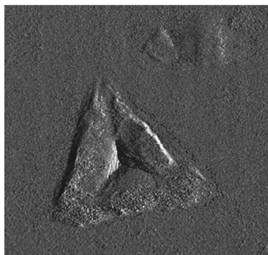
Figure 9. AFM picture of a Berkovich indent that was done on (top) 296 Å \text{HfO}_2 and (bottom) 104 Å \text{HfO}_2 thin films. The increase in roughness with film thickness can be seen.
