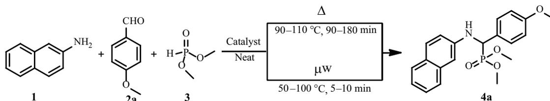
**Scheme 1.** Preparation of dimethyl ((4-methoxyphenyl)(naphthalen-2-ylamino)methyl)phosphonate (**4a**).
