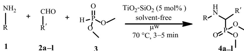
**Scheme 2.** Solvent-free microwave synthesis of  $\alpha$ -aminophosphonates (**4a–l**) on solid supported  $\text{TiO}_2\text{-SiO}_2$  catalyst.
