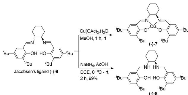
**Scheme 2.** Synthesis of (-)-**7**/copper (II) complex and tetrahydrosalen ligand (-)-**8** from (-)-**6**.
