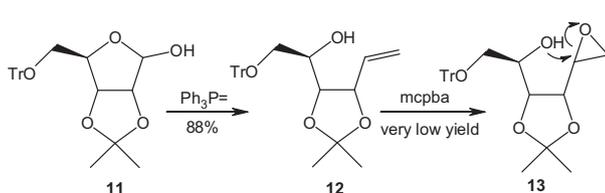
Scheme 1. Attempted synthesis of 1'-homologated nucleoside core. Reagents and conditions: (a) methyltriphenylphosphonium bromide, <sup>n</sup>BuLi, THF,  $-78\text{ }^{\circ}\text{C}\rightarrow\text{rt}$ , 16 h; (b) *m*-CPBA, DCE, reflux.
