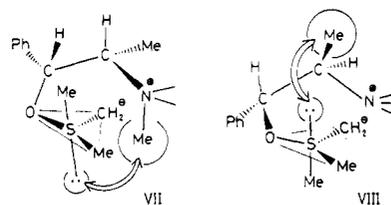
Less severe non-bonded interaction in the preferred conformer of skew boat type.
