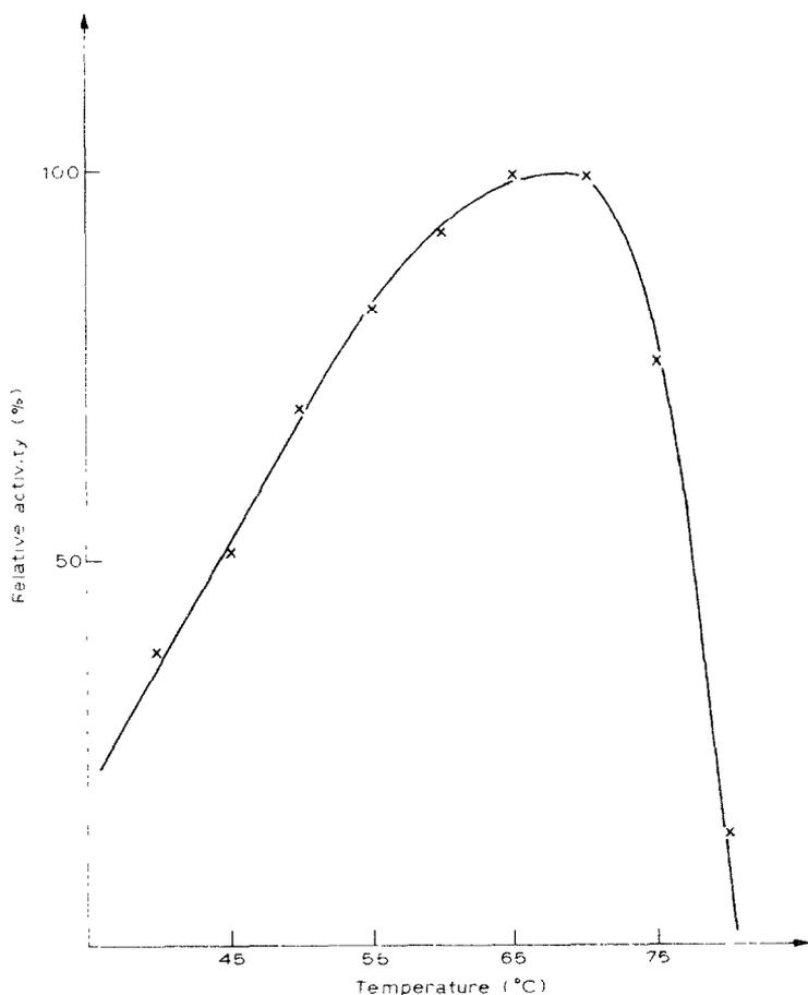
Fig. 5. Effect of temperature on the enzymic activity against xylan in 0.1M acetate buffer at the optimum pH of action. The test tubes containing both buffer and substrate were equilibrated for 10 min at the temperature investigated. Incubation with the xylanase was then performed as previously described for the assays. The curve is given for xylanase of pI 4.7.
