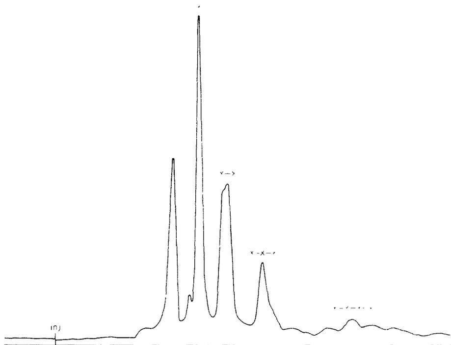
Fig. 7. L.c. analysis of the dialyzable products from the hydrolysis of xylan by pI 5.5 xylanase. The experiment was performed with a Waters liquid chromatograph using a  $C_{18}$   $\mu$ -Bondapak column kept at 20° and eluted with distilled water at the flow rate of 0.5 mL  $\text{min}^{-1}$ . The dialyzate was desalted on Amberlite IR-120 resin prior to injection. The xylo-oligosaccharide markers were isolated by filtration on Bio-Gel P-2 of an enzymic hydrolyzate of xylan.
