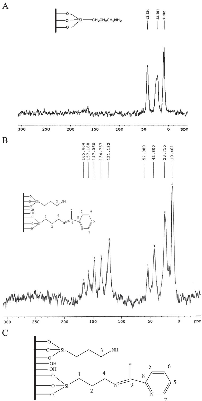
**Fig. 2.** a)  $^{13}\text{C}$  CP MAS NMR spectrum of aminopropyl silica gel (SG-NH<sub>2</sub>). b)  $^{13}\text{C}$  CP MAS NMR spectrum of ligand grafted silica gel (SG-NH<sub>2</sub>-AcPy). c) Labelling of carbon atoms in SG-NH<sub>2</sub>-AcPy in order of the peaks obtained in the spectrum of panel b.
