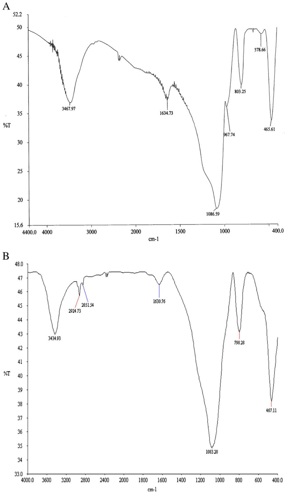
Fig. 1. FTIR spectra of a) silica gel (SG) b) aminopropyl silica gel (SG-NH<sub>2</sub>) c) ligand grafted silica gel (SG-NH<sub>2</sub>-AcPy).
