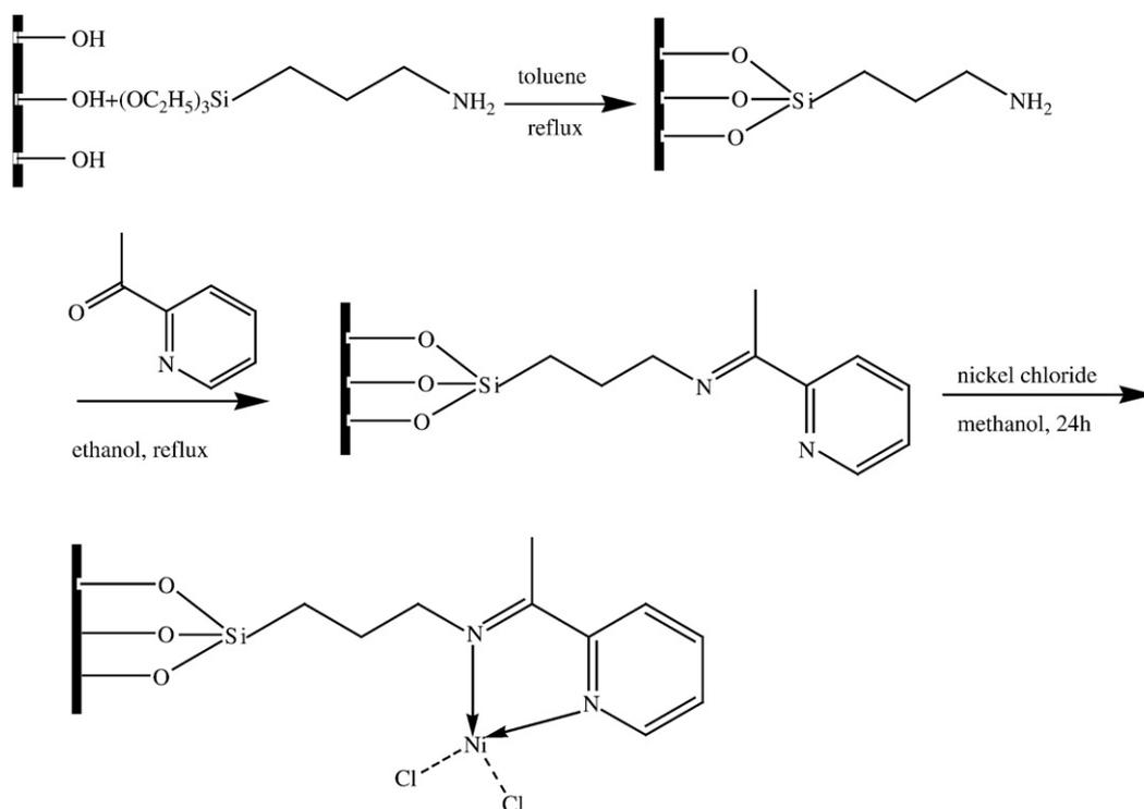
**Scheme 1.** Synthesis of covalently anchored nickel complex onto functionalized silica.
