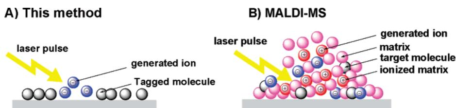
FIGURE 2. Schematic comparison of ionization process between tagged LDI-MS (A) and MALDI-MS (B).
