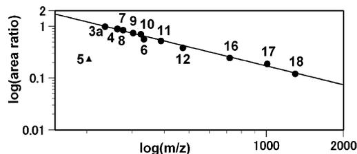
**FIGURE 1.** Dependence of relative response factors on molecular masses. Sensitivity of each compound was expressed as a ratio of signal area to **3a**. The values are average of ten spectra. An empirical equation was obtained by least-square method as  $y = 725.04x^{-1.208}$ ,  $R^2 = 0.991$ .
