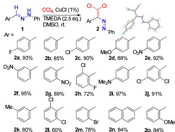
**Scheme 3. Scope of arylaldehyde hydrazones and molecular structure of 2a.**
