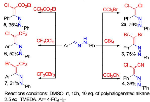
Reactions conditions: DMSO, rt, 10h, 10 eq. of polyhalogenated alkane, 2.5 eq. TMEDA. Ar = 4-FC<sub>6</sub>H<sub>4</sub>.
