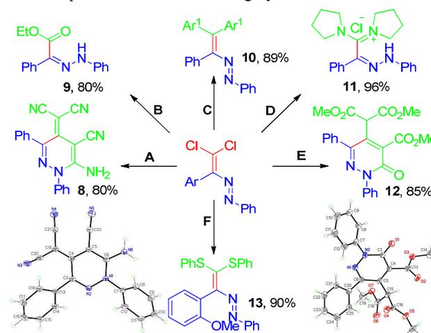
Reaction conditions A: CH<sub>2</sub>(CN)<sub>2</sub>, NaH, THF, rt, 5h. B: EtOH, reflux, 2h. C: Ar<sup>1</sup>=4-EtOC<sub>6</sub>H<sub>4</sub>-. Suzuki reaction, Ar<sup>1</sup>B(OH)<sub>2</sub>, S-Phos, K<sub>3</sub>PO<sub>4</sub>, toluene, rt, 6h. D: pyrrolidine, THF, rt, 5h. E: dimethyl malonate, NaH, THF, rt, 5h. F: PhSH, NaH, THF, rt, 6h.
