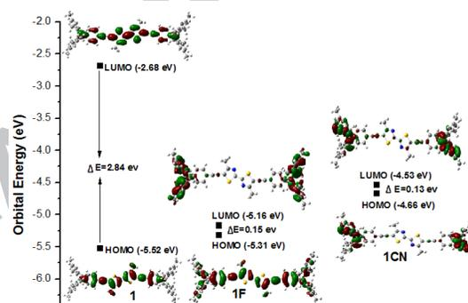
Fig 6. The energy level diagram of the frontier molecular orbitals of bisthiazole triarylborane dyad **1**, **1-F** and **1-CN** calculated using B3LYP level of TD-DFT theory.
