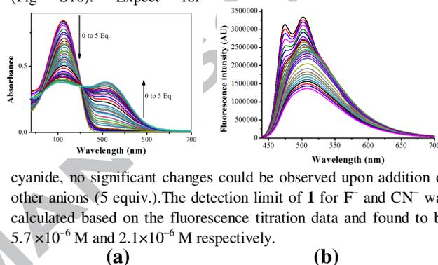
**Fig 3.** (a) Absorption and (b) fluorescence titration spectra of bisthiazole triarylborane **1** ( $2.1 \times 10^{-5}$  M) with TBACN in THF solvent.
