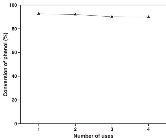
Fig. 5. Reusability of 8 wt.% TPAV<sub>1</sub>/SiO<sub>2</sub> catalyst.
