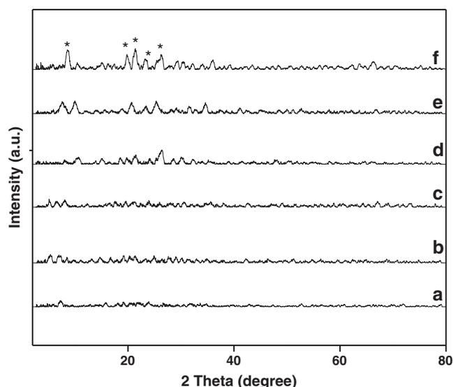
**Fig. 3.** XRD patterns of silica supported TPAV<sub>1</sub> catalysts. (a) 5 wt.% TPAV<sub>1</sub>/SiO<sub>2</sub> (b) 8 wt.% TPAV<sub>1</sub>/SiO<sub>2</sub> (c) 10 wt.% TPAV<sub>1</sub>/SiO<sub>2</sub> (d) 12 wt.% TPAV<sub>1</sub>/SiO<sub>2</sub> (e) 15 wt.% TPAV<sub>1</sub>/SiO<sub>2</sub> (f) 20 wt.% TPAV<sub>1</sub>/SiO<sub>2</sub>; TPAV<sub>1</sub> (·).
