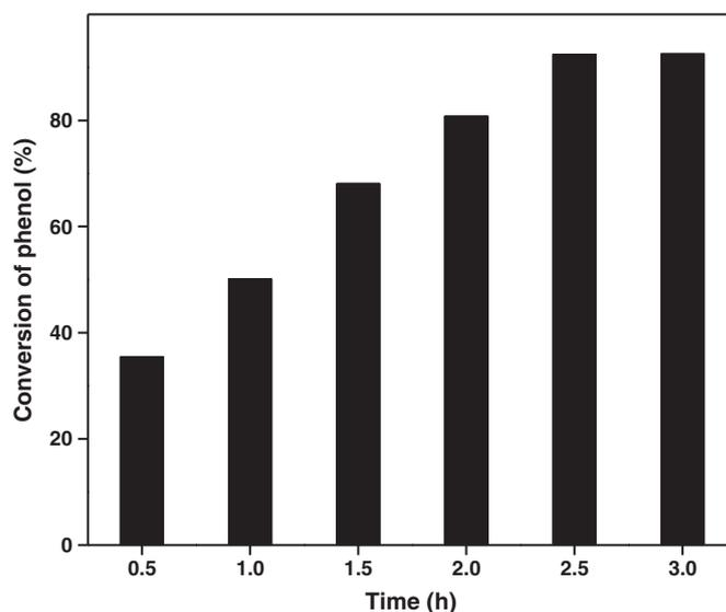
**Fig. 4.** Effect of reaction time on conversion of phenol.
