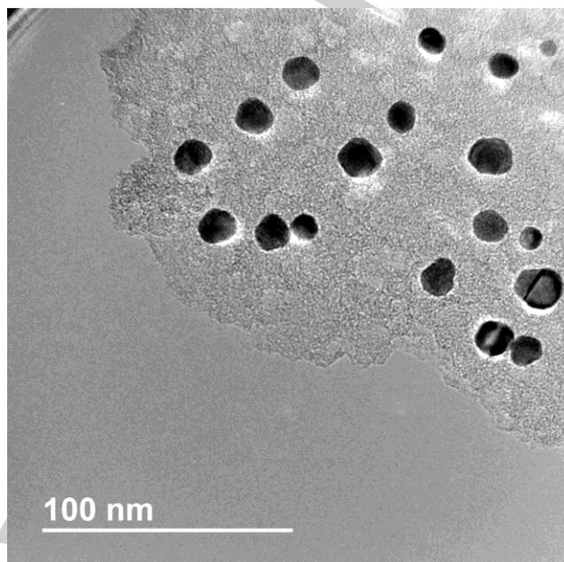
Figure 1. TEM image of the  $\text{Au}^{\text{fl-G}}/\text{Cu}_2\text{O}^{\text{fl-G}}$  catalyst.
