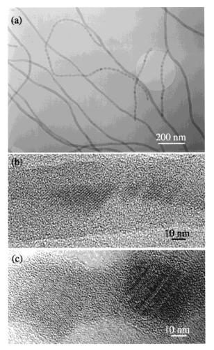
**Figure 10.** (a) TEM images of the Si nanowires formed in zone IV, showing two major morphologies. One is Si core sheathed with an amorphous silicon oxide outer layer (b); the other is chains of Si particles with different orientation (c).
