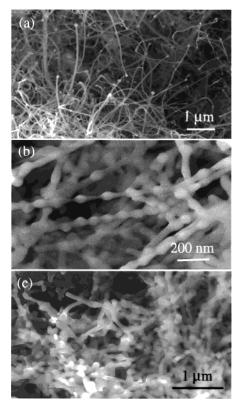
**Figure 5.** SEM images of the products formed in zone II. A yellow circular hard shell was formed in this zone inside the growth tube. The surface of the hard shell was composed of numerous pinlike nanowires (a), while the cross section of the shell was composed of sintered particle chains (b) and short bars (c).
