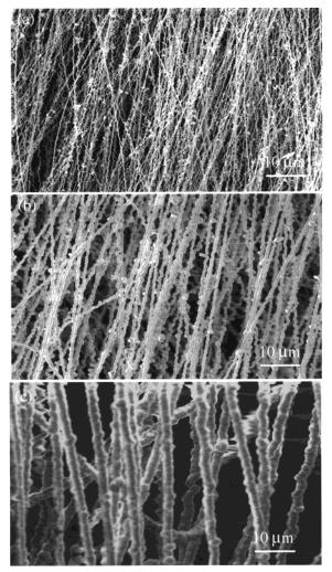
**Figure 11.** SEM images of the products formed in zone V. The products formed in this zone are light brown (a), brown (b), and dark brown (c) amorphous SiO wires (from high temperature to low temperature).
