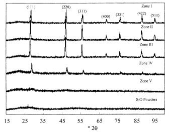
Figure 12. XRD spectra of the products formed in zones I-V, as well as the source material SiO powders.
