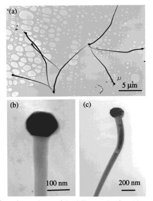
**Figure 6.** TEM images of the pinlike nanowires formed in zone II. The pinlike wires have a round tip and a sharp tail (a). The tip is crystalline Si, while the wire is either amorphous (b) (for thin wires) or a Si core sheathed with silicon oxide layer (c) (for thick wires).
