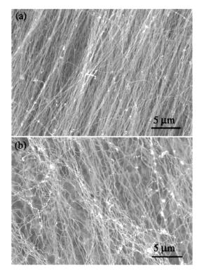
**Figure 9.** SEM images of the products formed in zone IV. The products formed in this zone are light yellow (a) and white yellow (b) Si nanowires, which grow along the flowing direction of the carrier gas and form quasi-aligned structures.
