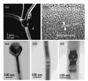
**Figure 4.** TEM and HRTEM images of the products formed in zone I. (a) Dark field TEM image of a octopuslike structure. (b) HRTEM image of the arm of the octopuslike structure shown in (a). (c) TEM image of the pinlike structure. TEM images of the Si nanowire with uniform Si core (d) and bulblike Si core (e).
