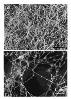
**Figure 7.** SEM images of the products formed in zone III. The color of the products formed in this zone is yellow mixed with pink. The yellow product is composed of very fine pinlike nanowires (a), while the pink product is composed of tadpolelike nanostructures (b).
