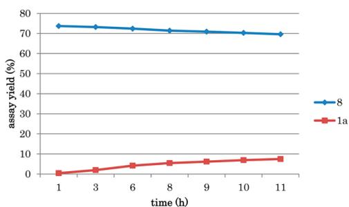
With regard to solubility after the reaction, assay yield was maintained at more than 70% for 10 h.<sup>14</sup> It was observed that the loss of assay yield was not caused by precipitation of **1b** but was a result of deacetylation of **1a**. **1a** is a target product in the deacetylation step, and including **1a** is not critical issue. It was desirable not to change the filtration property in filtering **1b** by including **1a** because **1a** showed poor filterability.
