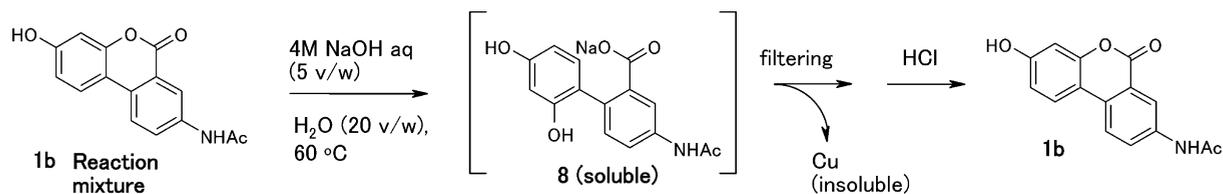
reaction suspension was also able to solve all components other than copper, which could be removed by cellulose powder pad filtration.<sup>13</sup> In 100 kg scale manufacturing, it was confirmed that residual copper is 4 ppm. Thus, **1b** was obtained under acidic conditions.
