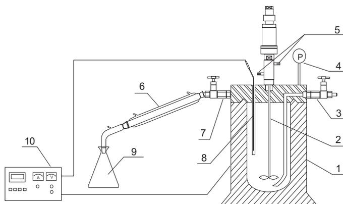
**Figure 9.** The schematic diagram of the experimental setup. (1) Stainless steel autoclave; (2) magnetic stirrer; (3) liquid bleed valve; (4) pressure gauge; (5 and 6) condenser; (7) vapor bleed valve; (8) thermocouple; (9) measuring receiver; (10) intelligent temperature controller.
