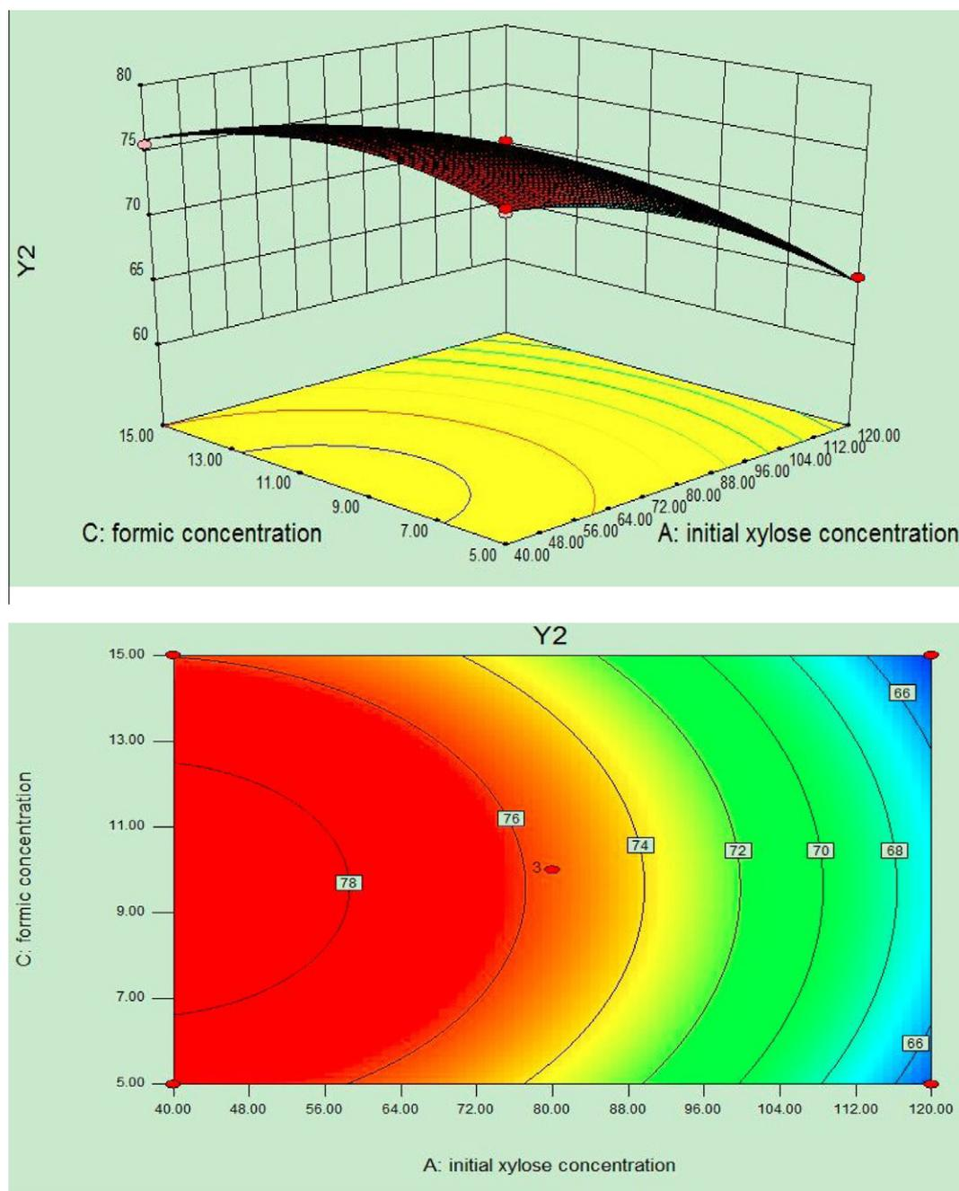
**Figure 8.** Effect of initial xylose concentration and formic concentration on furfural selectivity when temperature was set at 180 °C as the center point.
