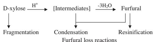
Scheme 1. Simplified scheme of the possible reaction in the xylose-to-furfural process.
