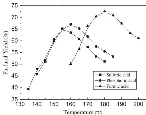
**Figure 3.** Dependence of furfural yield on reaction temperature with initial xylose concentration 80 g/L for different catalyst.
