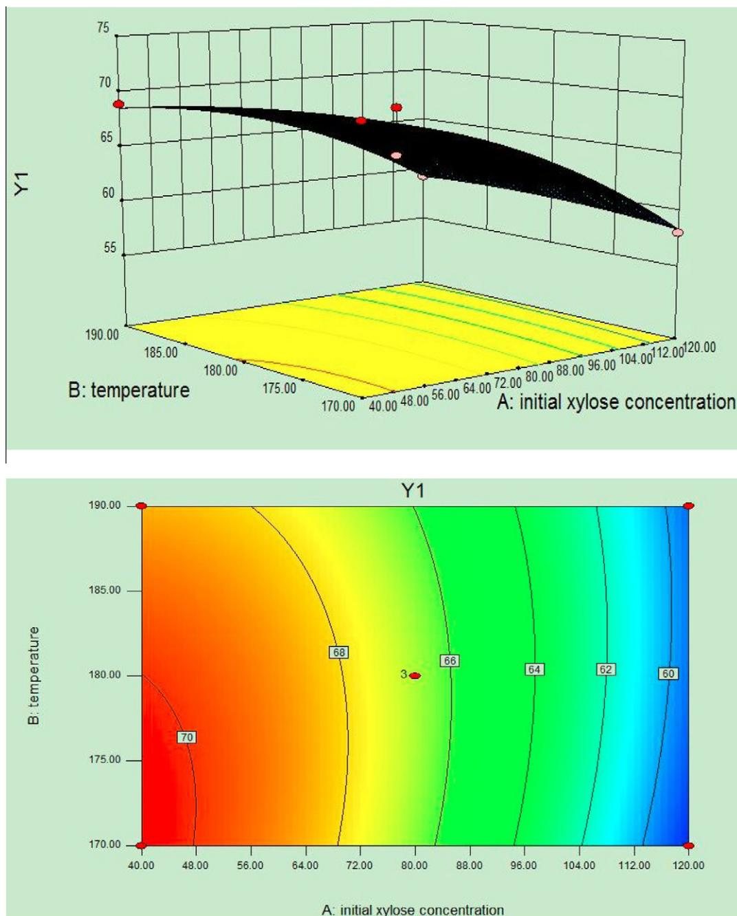
Figure 5. Effect of initial xylose concentration and temperature on furfural yield when formic concentration was set at 10 g/L as the center point.
