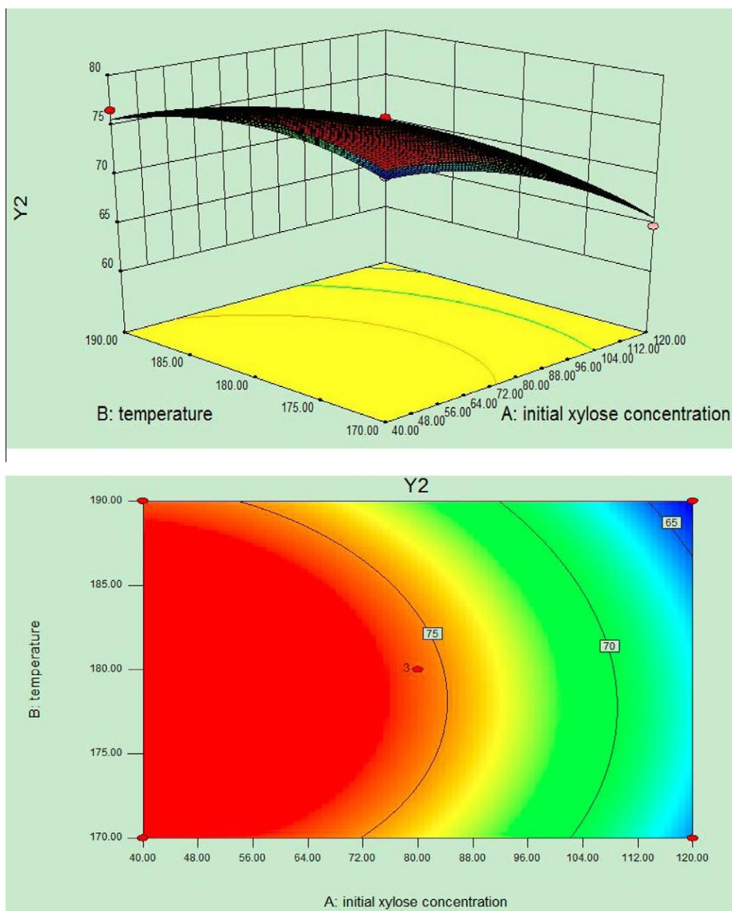
Figure 7. Effect of initial xylose concentration and temperature on furfural selectivity when formic concentration was set at 10 g/L as the center point.
