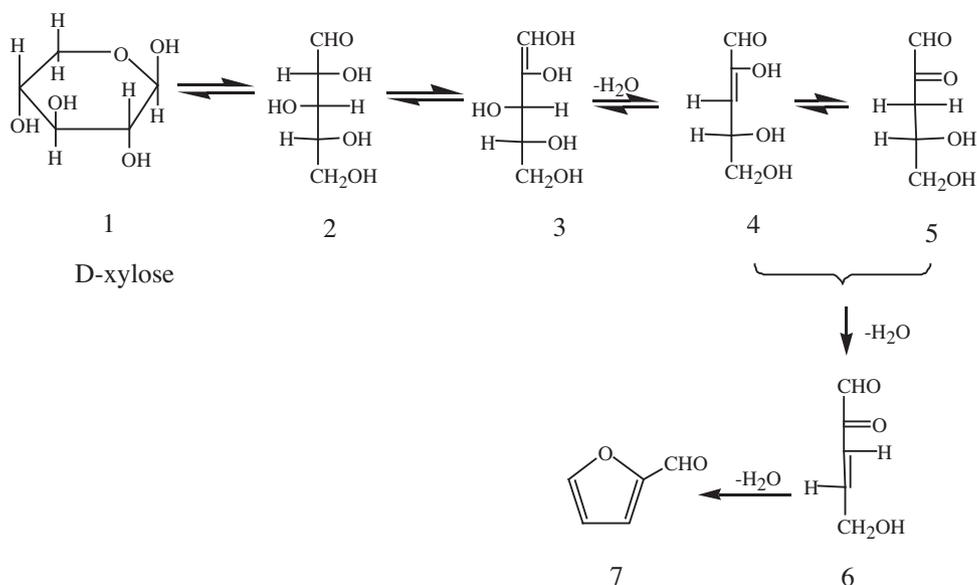
Figure 1. Mechanism (I) of the formation of 2-furfural from D-xylose.<sup>13</sup>
