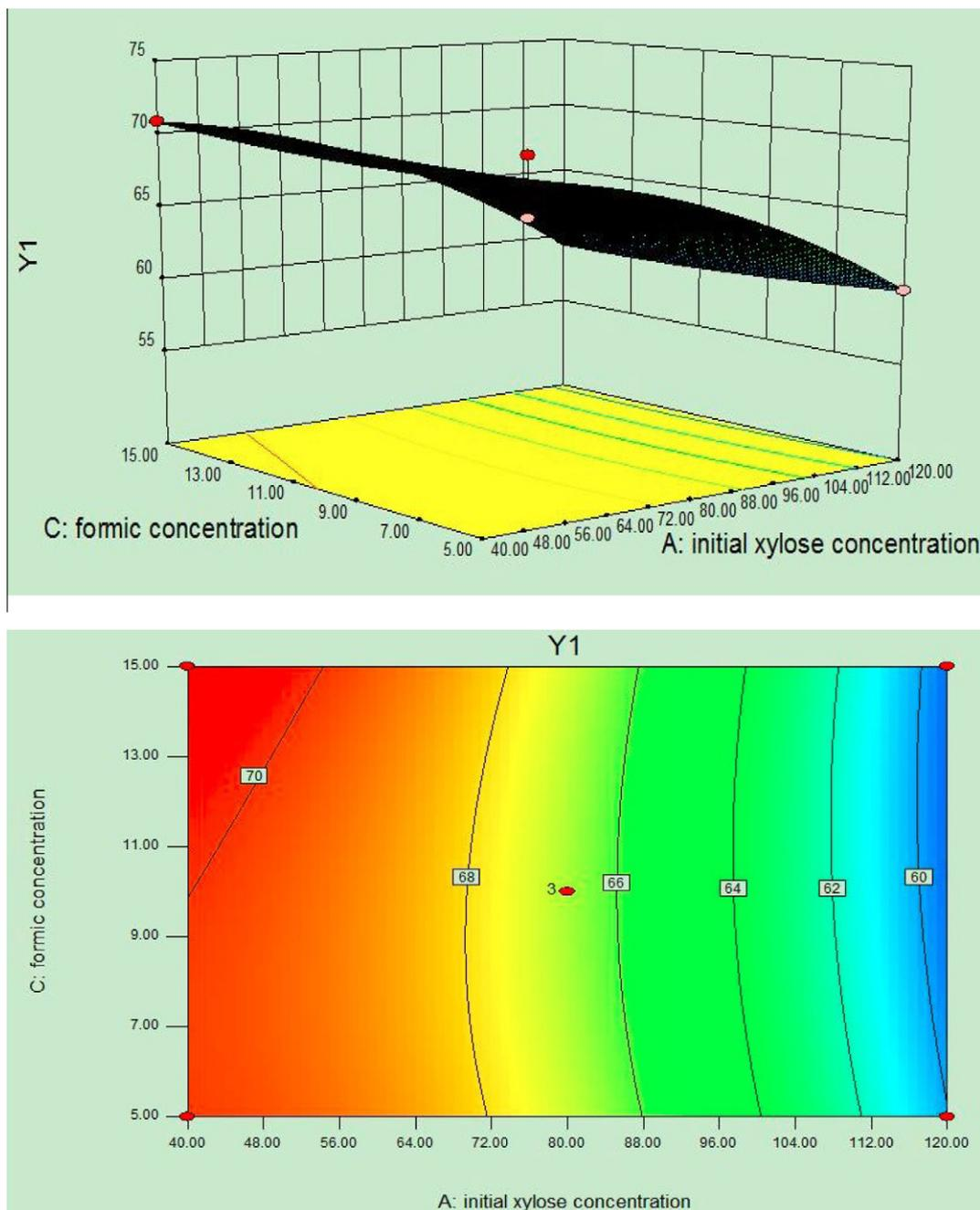
Figure 6. Effect of initial xylose concentration and formic concentration on furfural yield when temperature was set at 180 °C as the center point.
