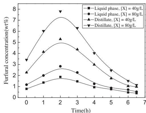
**Figure 4.** The furfural concentrations of distillate and liquid phases in the autoclave at different time with 15 g/L formic acid.
