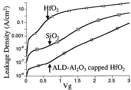
FIG. 4.  $I$ – $V$  data for similar electrical thickness films with 620 °C LPCVD Si-gate and HfO<sub>2</sub>, SiO<sub>2</sub>, or ALD–Al<sub>2</sub>O<sub>3</sub> capped HfO<sub>2</sub> dielectrics.
