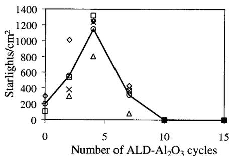
FIG. 3. Density of observed starlight inhomogeneous grains vs the number of ALD–Al<sub>2</sub>O<sub>3</sub> cycles (1 cycle = TMA pulse + H<sub>2</sub>O pulse).
