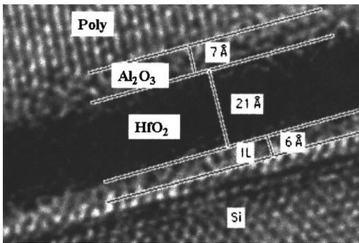
FIG. 2. XTEM of the poly-Si/Al<sub>2</sub>O<sub>3</sub> capped HfO<sub>2</sub> gate stack after a 1000 °C 30 s anneal.
