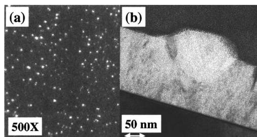
FIG. 1. (a) Dark-field optical image (500 $\times$ ) showing observed poly-Si starlight inhomogeneous grain growth. (b) Cross-sectional (XTEM) of a poly-Si starlight grain.
