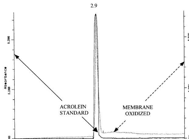
**Figure 4** Superposition of two electropherograms corresponding to an acrolein standard and the peak corresponding to the product of the oxidation of erythrocyte membranes with ozone. The migration time of the two peaks was equal or very proximate between the two successive assays. A selected electropherogram is shown
