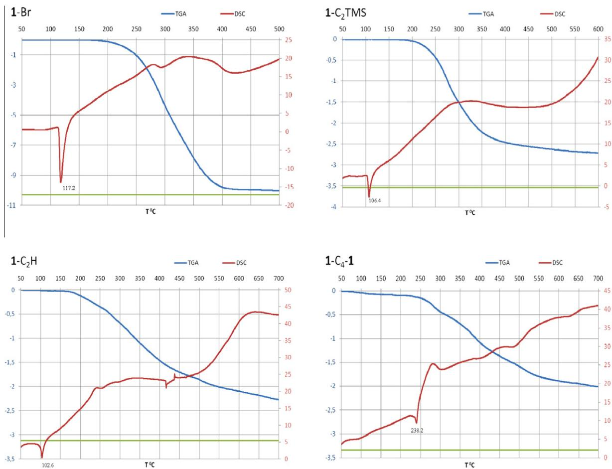
Figure 2. DSC for benzoxazines: **1-Br** (top, left), **1-C<sub>2</sub>TMS** (top, right), **1-C<sub>2</sub>H** (bottom, left), and **1-C<sub>4</sub>-1** (bottom, right).
