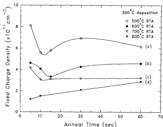
Fig. 7. Fixed charge density as a function of anneal time, for samples deposited at  $300^\circ\text{C}$  (a)  $500^\circ\text{C}$ , (b)  $600^\circ\text{C}$ , (c)  $700^\circ\text{C}$ , and (d)  $800^\circ\text{C}$  anneals.
