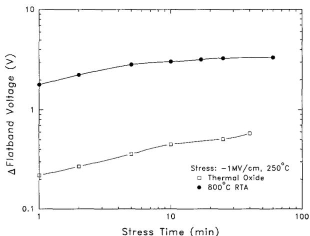
Fig. 9. Change in flatband voltage as a function of stress period. The sample was deposited at  $300^\circ\text{C}$  and annealed at  $800^\circ\text{C}$  for 5 s. The stress temperature was  $250^\circ\text{C}$  and stress field was  $1 \text{ MV/cm}$ .
