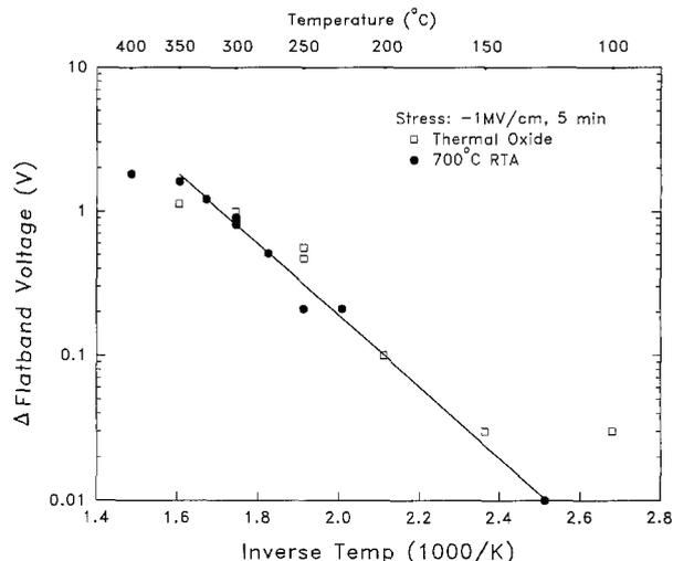
Fig. 8. Change in flatband voltage as a function of stress temperature. The sample was deposited at  $300^\circ\text{C}$  and annealed at  $700^\circ\text{C}$  for 5 s. The stress period was 5 min and the stress field was  $+1 \text{ MV/cm}$ .
