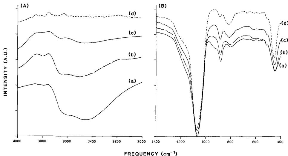
tion of a small amount of silanol groups present. Note the strong bands at approximately 1058, 812, and 450 cm<sup>-1</sup> for the 300°C sample, due to Si-O bond stretching, bending, and rocking modes, respectively. Thus, as the deposition temperature is raised, less water is found in the films, they become more stoichiometric, and the bands become closer to those of thermal oxide (17).
