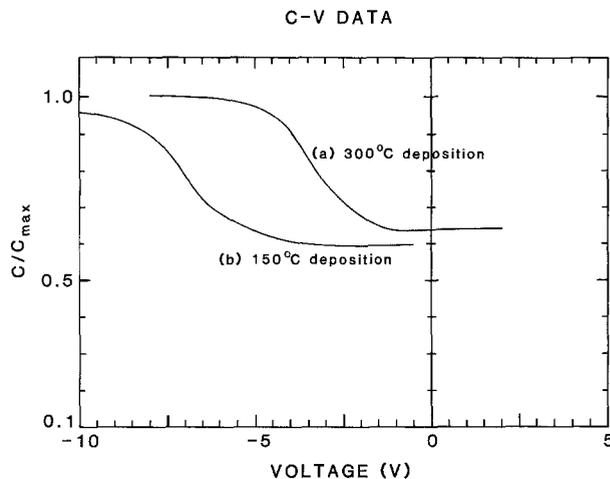
Fig. 4. 1 MHz capacitance-voltage data. (a) 300°C, 3 Torr, 8 min deposition,  $d_{ox} = 1437 \text{ \AA}$ , (b) 150°C, 4 Torr, 15 min deposition,  $d_{ox} = 1409 \text{ \AA}$ .
