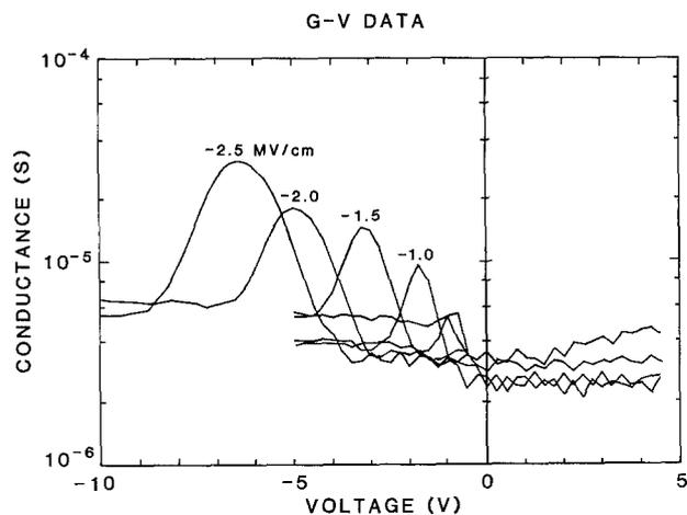
Fig. 10. Conductance-voltage data as a function of stress field. The sample was deposited at 300°C and annealed at 800°C for 5 s. The stress temperature was 200°C and stress time was 5 min.
