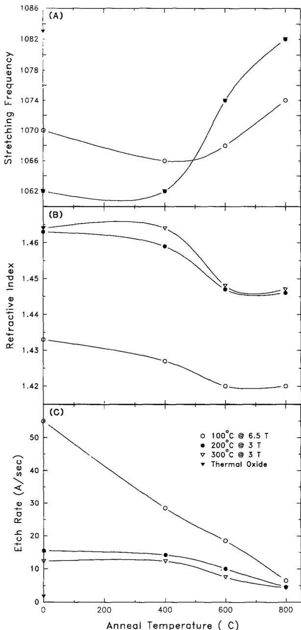
Fig. 3. The effect of annealing on a) Si-O stretching frequency, b) refractive index, and c) P-etch rate.
