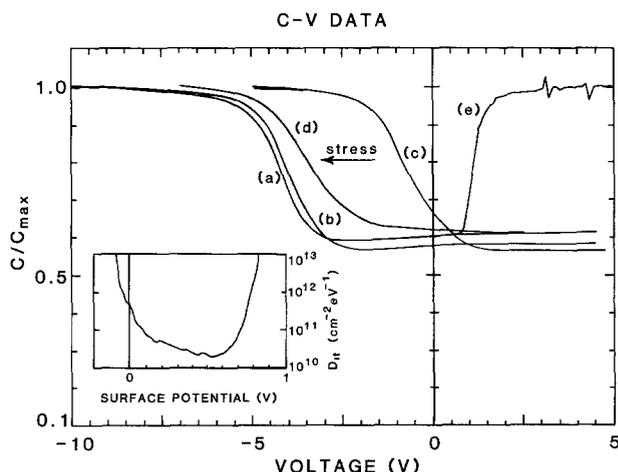
Fig. 6. Capacitance-voltage data for sample deposited at 300°C. (a) deposited, (b) after stress, (c) 800°C, 5 s RTA, (d) annealed sample after stress, (e) quasi-static data for annealed sample. Insert is  $D_{it}$  calculation using the high and low frequency data of (c) and (e).
