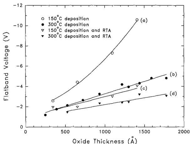
Fig. 5. Flatband voltage as a function of oxide thickness. (a) 300°C deposition, (b) 300°C samples after 650°C, 15 s RTA. (c) 150°C deposition, (d) 150°C samples after 650°C, 15 s RTA.
