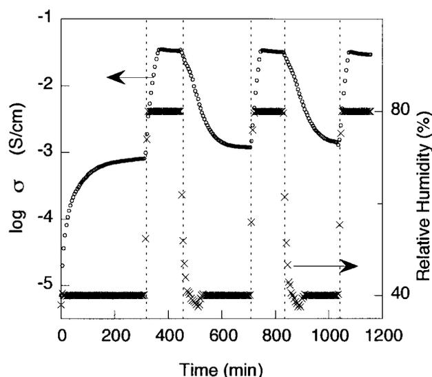
Fig. 6. Change in conductivity, measured at  $50^\circ C$ , on exposure to humid atmospheres of 40% and 80%.
