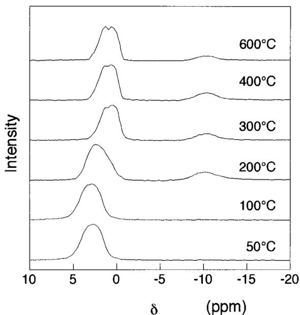
**Fig. 2.** P-MAS-NMR spectra of the 5P<sub>2</sub>O<sub>5</sub>·95SiO<sub>2</sub> glasses obtained by heating at 50° to 600°C using PO(OCH<sub>3</sub>)<sub>3</sub>.
