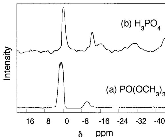
Fig. 1. P-MAS-NMR spectra of the 5P<sub>2</sub>O<sub>5</sub>·95SiO<sub>2</sub> glasses obtained by heating at 600°C using PO(OCH<sub>3</sub>)<sub>3</sub> and H<sub>3</sub>PO<sub>4</sub>.
