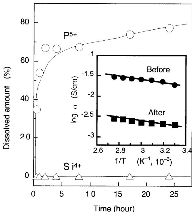
Fig. 5. Dependence of the dissolved amount of  $P^{5+}$  and  $Si^{4+}$  ions on the immersion time in water for the  $5P_2O_5 \cdot 95SiO_2$  glasses heated at  $600^\circ C$ . Inset indicates the temperature dependence of conductivity of the glass before and after immersion for 24 h.
