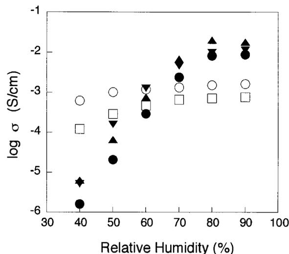
**Fig. 3.** Relation between the conductivity, measured at 30°C, and the relative humidity for the 5P<sub>2</sub>O<sub>5</sub>·95SiO<sub>2</sub> glasses heated at 50° (○), 100° (□), 300° (●), 400° (▲), and 500° (▼).
