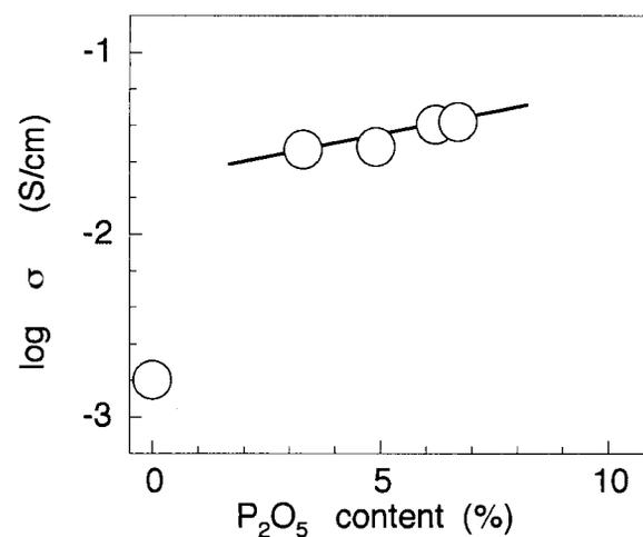
**Fig. 4.** Relation between the conductivity, measured at 30°C under 70% RH, and the content of P<sub>2</sub>O<sub>5</sub> in the glasses heated at 600°C.
