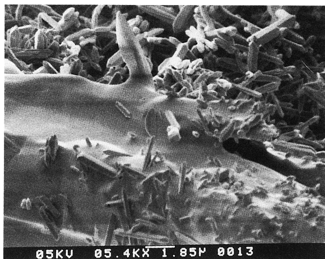
Fig. 8. Incomplete pyrolysis of fluorotopaz showing metastable melt.
