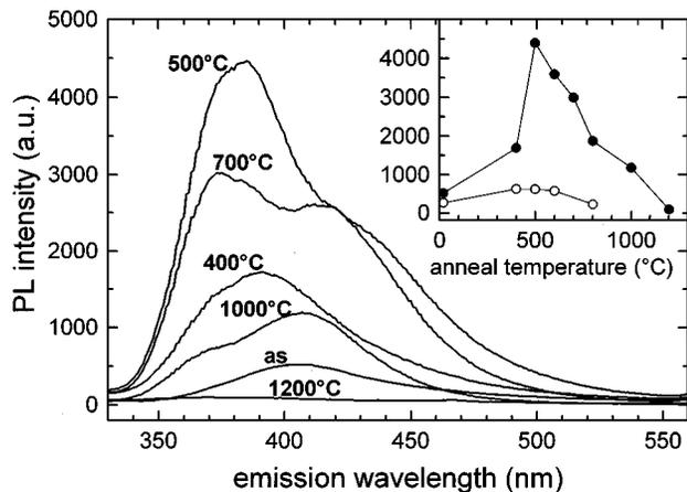
FIG. 1. The PL spectra from Ge-implanted  $\text{SiO}_2$  films after implantation (as) and at different anneal temperatures under 240 nm excitation. The inset shows the PL intensity maximum from both Ge- (closed circles) and Si- (open circles) implanted  $\text{SiO}_2$  films depending on anneal temperature.
