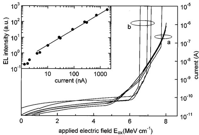
FIG. 3. The dependence of injection current on the applied electrical field  $E_{ox}$  for Ge-rich  $\text{SiO}_2$  furnace-annealed at  $1000\text{ }^\circ\text{C}$  (a) and pure oxide (b). The inset shows the EL intensity for the Ge-implanted  $\text{SiO}_2$  films as a function of current. The solid line represents a linear fit between  $3.9\text{ nA}$  and  $1.8\text{ }\mu\text{A}$ .
