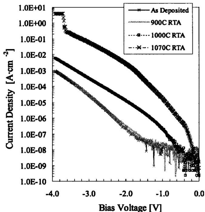
**Figure 8.** I-V characteristics of SiO<sub>2</sub>-rich HfSiO<sub>4</sub> layers for various polysilicon anneals (same layer as in Fig. 7).
