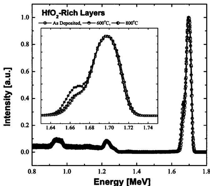
**Figure 3.** RBS measurements of HfO<sub>2</sub>-rich silicate layers with various PDAs.
