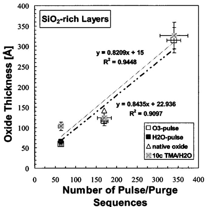
**Figure 1.** Thickness of  $\text{SiO}_2$ -rich silicate layers for various starting conditions. Average growth per pulse/purge sequence is 0.82-0.84 Å/pulse/purge sequence.
