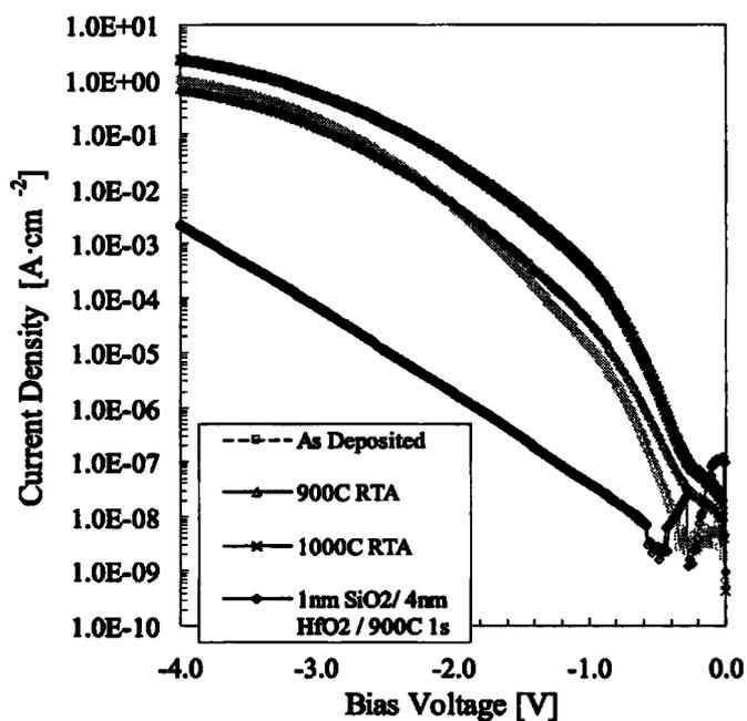
**Figure 10.** I-V measurements of HfO<sub>2</sub>-rich HfSiO<sub>4</sub> layer on Al<sub>2</sub>O<sub>3</sub> start surface, including reference data of 4 nm HfO<sub>2</sub>.
