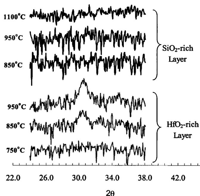
Figure 5. XRD results for HfO<sub>2</sub>-rich and SiO<sub>2</sub>-rich layers.
