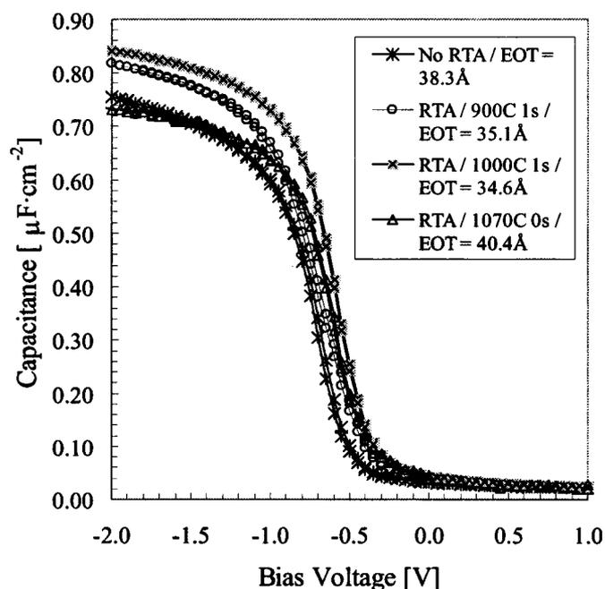
**Figure 7.** C-V characteristics of SiO<sub>2</sub>-rich HfSiO<sub>4</sub> (64 cycles 1:1 with O<sub>3</sub> start pulse) for various polysilicon anneals (silicate layer is as-deposited). EOTs range from 38.3 (as-deposited) to 40.4 Å (1070°C spike anneal).
