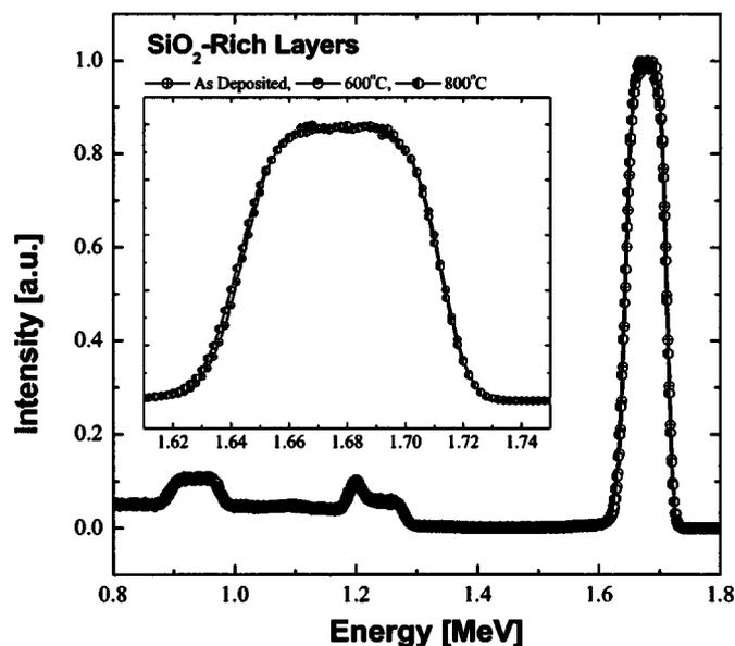
**Figure 4.** RBS measurements of SiO<sub>2</sub>-rich silicate layers which received as-indicated PDAs.
