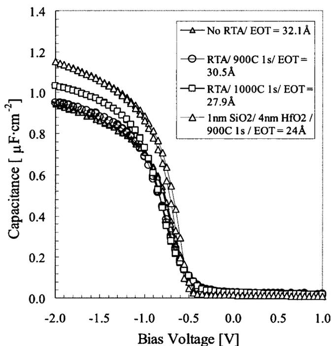
**Figure 9.** C-V measurements of HfO<sub>2</sub>-rich layer on Al<sub>2</sub>O<sub>3</sub> start surface, including reference HfO<sub>2</sub> with polysilicon after 900°C activation anneal.
