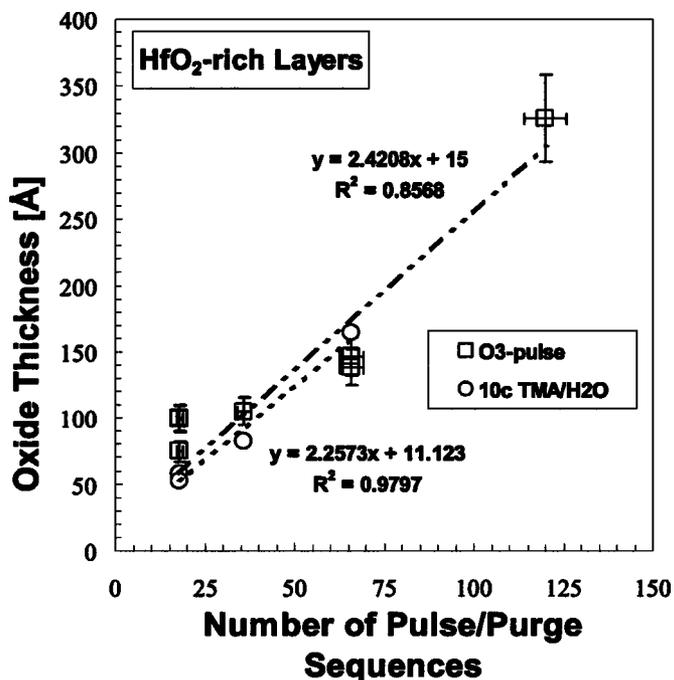
**Figure 2.** Thickness of  $\text{HfO}_2$ -rich silicate layers for various starting conditions. Average growth per pulse/purge sequence is 2.26-2.42 Å/pulse/purge sequence.
