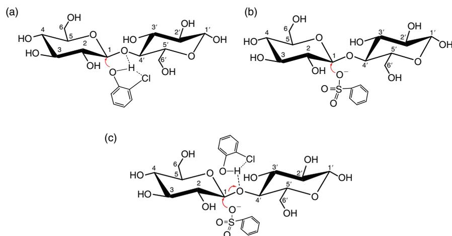
**Fig. 2.** Possible ways of attack of catalyst on cellobiose during hydrolysis: *o*-chlorophenol (a), sodium benzenesulfonate (b), and DMNC (c).
