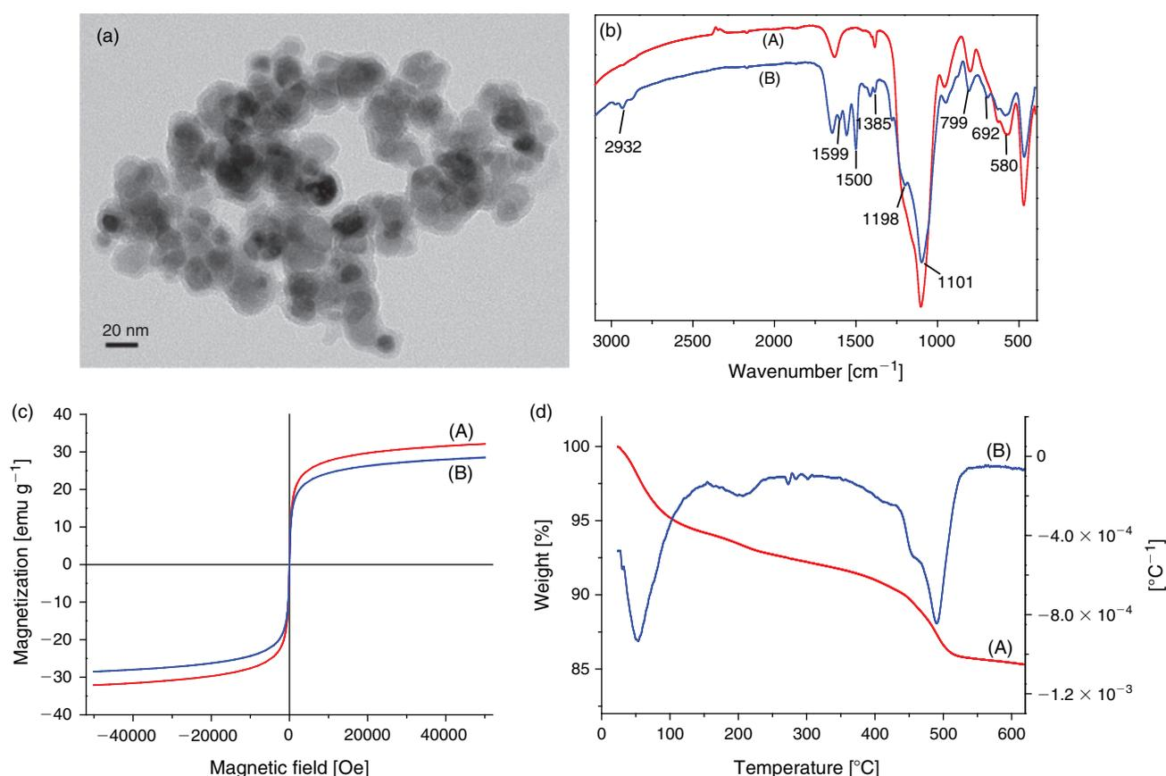
**Fig. 1.** (a) TEM images of DMNC; (b) FT-IR spectra of  $\text{Fe}_3\text{O}_4@\text{SiO}_2$  (A) and DMNC (B); (c) magnetic hysteresis loop of DMNC at 300 K (A) and 400 K (B); (d) TGA (A) and differential thermal gravimetric (DTG) analysis (B) curves of DMNC.
