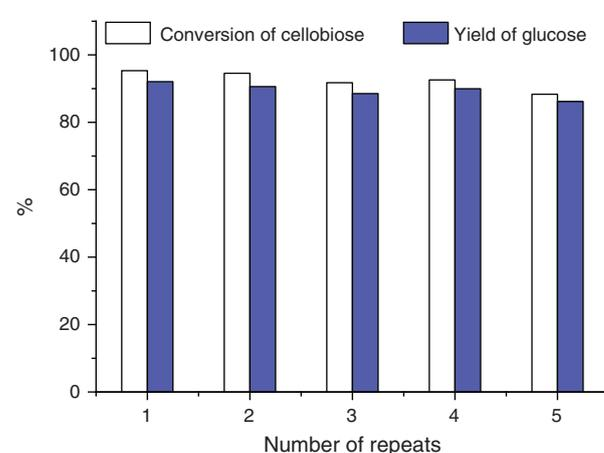
**Fig. 5.** DMNC cycle for cellobiose hydrolysis.
