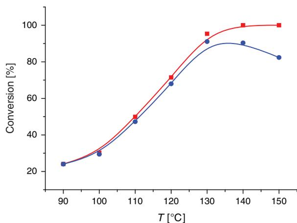
**Fig. 3.** Plots of conversion of cellobiose (■) and yield of glucose (●) versus reaction temperature, pH 4.0, 6 h.
