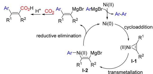
was reduced by Grignard reagents to deliver Ni(0), which undergoes cycloaddition with alkyne to give Ni(II) complex I-1. Then the aryl Grignard reagent triggers transmetalation to afford new Ni(II) complex I-2. Finally, reductive elimination takes place to generate the arylmagnesium-substituted alkene, which gives acrylic acid **3** after addition of CO<sub>2</sub> and hydrolysis.
