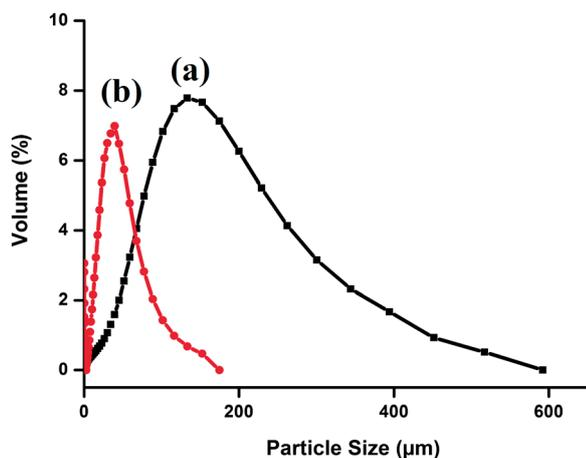
Fig. 4 Particle-size histograms: (a) biobased; (b) non-biobased PF microcapsules.
