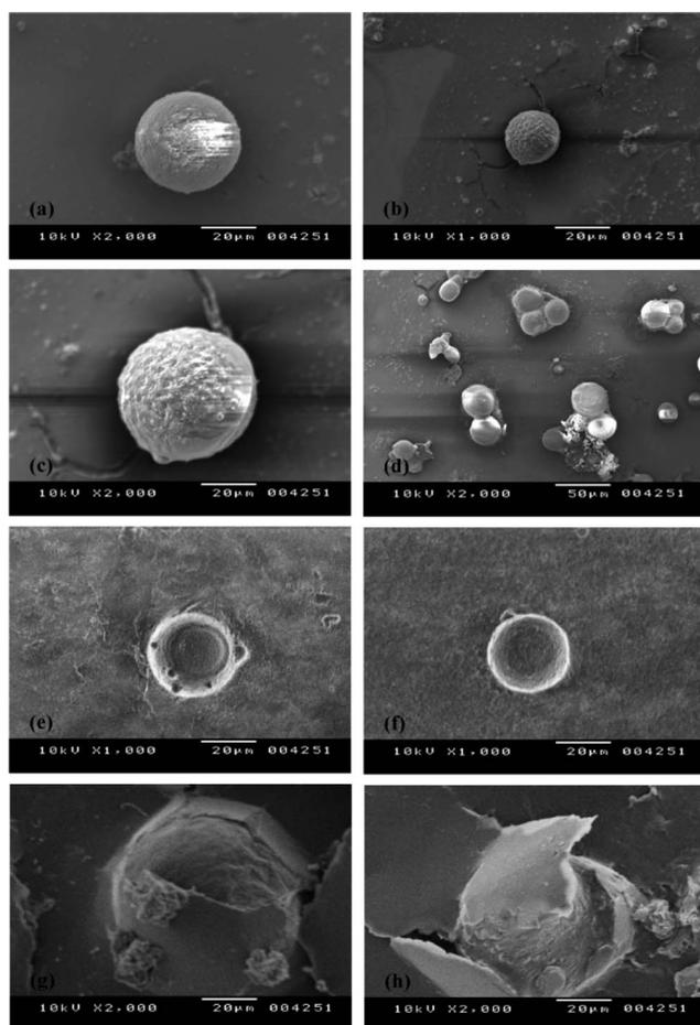
Fig. 2 SEM micrographs of biobased microcapsules exposed to  $50\text{ }^{\circ}\text{C}$  (a and b) 00 h, (c and d) 48 h, (e and f) 96 h and (g and h) 144 h.
