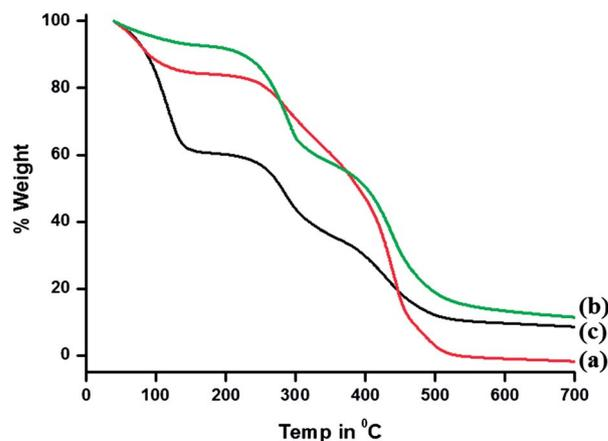
Fig. 5 TGA curves (a) cardanol-based novel microcapsules; (b) phenol–formaldehyde conventional microcapsules; and (c) core bio-pesticides.
