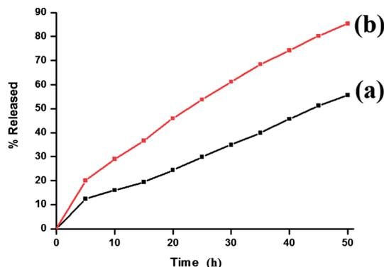
Fig. 6 Release rate from (a) biobased and (b) non-biobased microcapsules.
