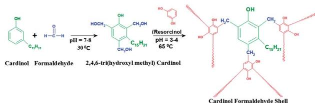
Fig. 1 Reaction scheme for renewable sources based on cardanol formaldehyde (CF) novel microcapsules.
