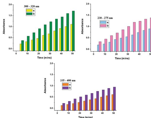
Fig. 7 UV plots for extracted core material: (a) biobased microcapsules; (b) conventional non-biobased microcapsules.
