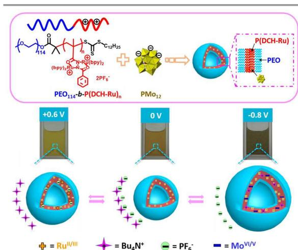
**Figure 1.** Schematic illustration of the hybrid co-assembly of cationic block copolymer  $\text{PEO}_{114}\text{-}b\text{-P(DCH-Ru)}_n$  with anionic Keggin polyoxometalate  $\text{PMo}_{12}$  and transmembrane transport process of different ions.
