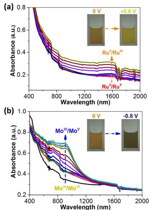
**Figure 2.** UV-vis-NIR absorption spectra and electrochromism of the coassemblies of  $\text{PEO}_{114}\text{-}b\text{-P(DCH-Ru)}_{14}/\text{PMo}_{12}$  in  $\text{CH}_3\text{CN}$  with 0.1 M  $\text{Bu}_4\text{NPF}_6$ .
