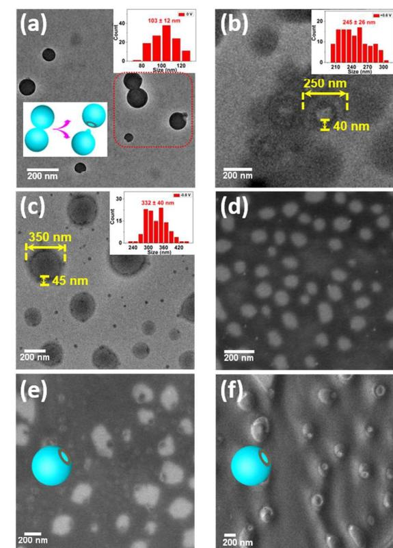
**Figure 3.** TEM images at (a) 0 V, (b) +0.6 V, (c) -0.8 V; SEM images at (d) 0 V, (e) +0.6 V, (f) -0.8 V state of the hybrid coassemblies PEO<sub>114</sub>-*b*-P(DCH-Ru)<sub>14</sub>/PMo<sub>12</sub>.
