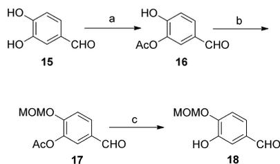
**Scheme 2.** a) Ac<sub>2</sub>O, NaOH, THF, 0°C, 82–85%; b) MOMCl, K<sub>2</sub>CO<sub>3</sub>, DMF, 0°C to RT, 76–80%; c) K<sub>2</sub>CO<sub>3</sub>, MeOH, RT, 88–90%. DMF = *N,N*-dimethylformamide.
