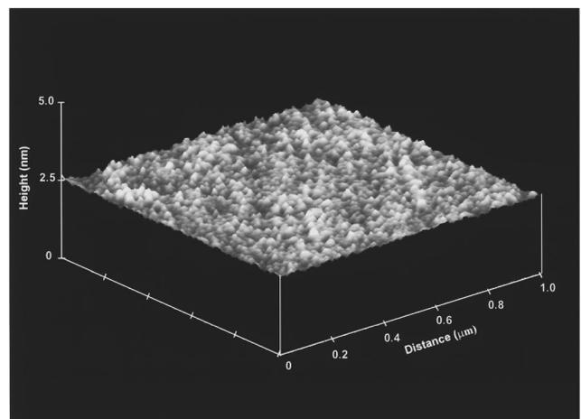
FIG. 3. Atomic force microscope image of a SiO<sub>2</sub> film deposited directly on Si(100) at 700 K after 75 AB cycles. The horizontal full scale is 1  $\mu$ m. The vertical full scale is 5 nm and the light-to-dark range is 10 Å.
