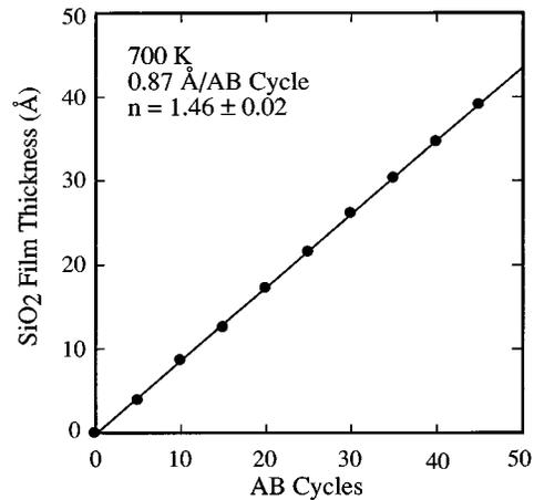
FIG. 2. Ellipsometric measurements of SiO<sub>2</sub> film thickness deposited on thin Al<sub>2</sub>O<sub>3</sub> films on Si(100) at 700 K vs number of AB reaction cycles.
