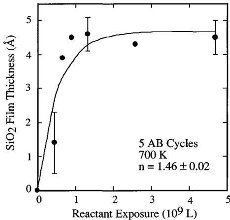
FIG. 1. Ellipsometric measurements of SiO<sub>2</sub> film thickness deposited on thin Al<sub>2</sub>O<sub>3</sub> films on Si(100) at 700 K after 5 AB cycles for various total reactant exposures.
