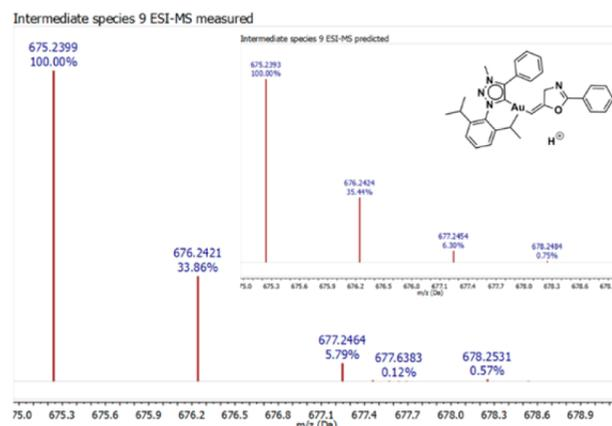
Figure 3. Measured and predicted ESI-MS for intermediate gold(I) MIC vinyl species **9**.
