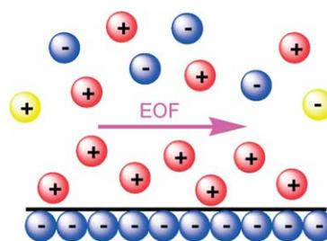
**Figure 6.** Schematic illustrating the principle of electroosmotic flow.
