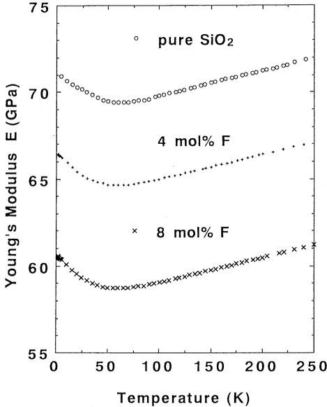
Fig. 2. Young's moduli of pure  $\text{SiO}_2$ ,  $\text{SiO}_2$ -4 mol% F and -8 mol% F glasses.
