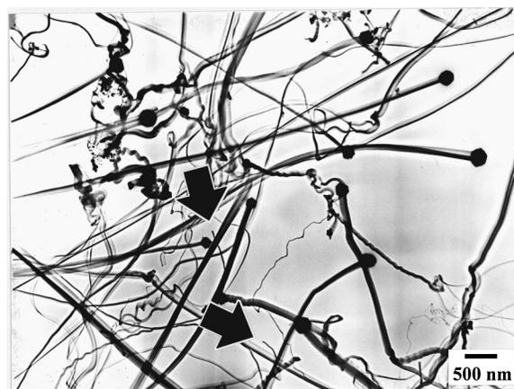
FIG. 4. TEM image of metallic catalysts on the tips of the nanowires.
