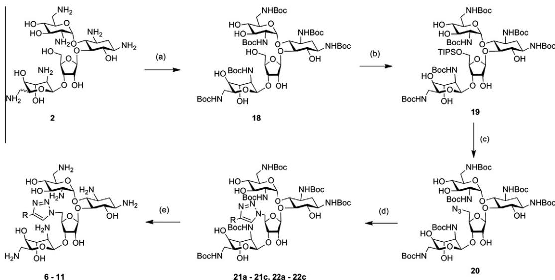
**Scheme 2.** Synthesis of conjugates **6–11**. Conditions: (a) Boc<sub>2</sub>O (10 equiv), TEA/MeOH/H<sub>2</sub>O (61%). (b) TIPS-Cl (31 equiv), pyridine (41%). (c) NaN<sub>3</sub> (10 equiv), DMF/H<sub>2</sub>O (94%). (d) **16a–c**, **17a–c** (1.2 equiv), CuI (0.2 equiv), DIPEA (3 equiv), ACN (50–88%). (e) TFA/H<sub>2</sub>O (80–91%).
